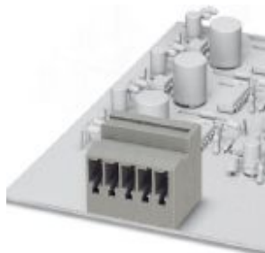
ST-COMBI receptacle, plug-in direction horizontal to the PCB, pitch: 6.2 mm, no. of positions: 5
