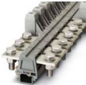
Universal terminal block with bolt connection, cross section: 35 ... 95 mm 2 , AWG: 2 ... 4/0, width: 40 mm, color: gray
