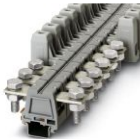
Universal terminal block with bolt connection, cross section: 25 ... 50 mm 2 , AWG: 6 ... 1/0, width: 32 mm, color: gray
