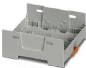
DIN rail housing, Lower housing part with base latch, flat design, width: 70.1 mm, height: 75 mm, depth: 30.3 mm, color: light gray (7035)
