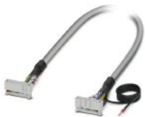
Assembled shielded round cable; connection 1: IDC/FLK socket strip (1x 14-position); connection 2: IDC/FLK socket strip (1x 14-position) (The braided shield is routed to a separate cable end.); cable length: 6 m
