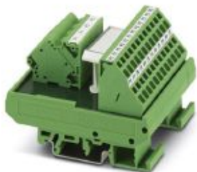
VARIOFACE module, with two equipotential busbars (P1, P2) for potential distribution, for mounting on NS 32 or on NS 35/7.5
