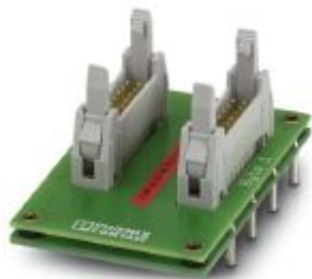
VARIOFACE front adapter for Inline modules, for transferring 16 (2 x 8) digital output signals.
