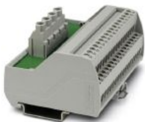
VARIOFACE module, with two equipotential busbars (P1, P2) for potential distribution, for mounting on NS 35 rails. Module width: 90.8 mm
