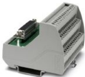
VARIOFACE module, with screw connection and high density D-SUB miniature socket strip, for mounting on NS 35 rails, no. of pos.: 44, width: 135 mm
