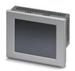
Touch panel with 14.5 cm/5.7" TFT active-display (analog resistive (polyester)), 640 x 480 Pixel(s) (VGA), 262144 colors, ARM® Cortex®-A8, 1000 MHz, 2x USB host 2.0, 1 x Ethernet (10/100 Mbps), RJ45, Debian GNU/Linux and user software: Firefox Browser. (bus system: without)
