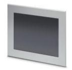
Touch panel with 26.4 cm/10.4" TFT-display (analog resistive (polyester)), 800 x 600 Pixel(s) (SVGA), 262144 colors, ARM® Cortex®-A8, 1000 MHz, 2x USB host 2.0, 1 x Ethernet (10/100 Mbps), RJ45, Debian GNU/Linux and user software: Firefox Browser. (bus system: without)
