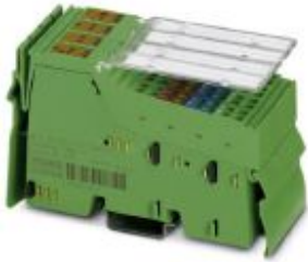
Inline IO-Link master, complete with accessories (connector and labeling field), 4 IO-Link ports, 12 digital inputs, 24 V DC, transmission speed 2 Mbaud, 2, 3-wire connection method
