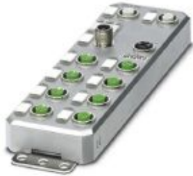
Axioline E PROFINET device in a metal housing with 8 IO-Link ports and 4 digital inputs, 24 V DC, M12 fast connection technology
