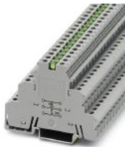
Sensor/actuator terminal block, connection method: Screw connection, cross section: 0.2 mm 2 - 4 mm 2 , AWG: 24 - 12, width: 6.2 mm, color: gray, mounting type: NS 35/7,5, NS 35/15
