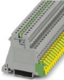
Sensor/actuator terminal block, connection method: Screw connection, cross section: 0.2 mm 2 - 4 mm 2 , AWG: 24 - 12, width: 6.2 mm, color: gray, mounting type: NS 35/7,5, NS 35/15
