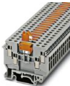
Knife disconnect terminal block with two-sided double connection, cross section: 0.2 - 2.5 mm 2 , AWG: 30 - 10, width: 6.2 mm, color: gray
