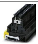
Modular terminal block with suppressor diode as surge voltage protection between clamping connector and DIN rail, separate ground connection, nominal voltage: 5 V AC, mounting on NS 35/7.5, terminal width: 6.2 mm, terminal height: 69 mm
