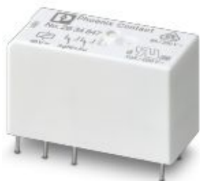
Plug-in miniature power relay, with multi-layer gold contact, 2 PDTs, input voltage 48 V DC
