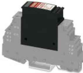
Type 3 arrester replacement connector (device protection) for 1-phase power supply networks with separate N and PE (3-conductor system: L1, N, PE).
