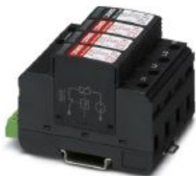
Surge voltage arrester 4-channel, for mounting on NS 35/7.5, with remote indicator contact. 350 V AC
