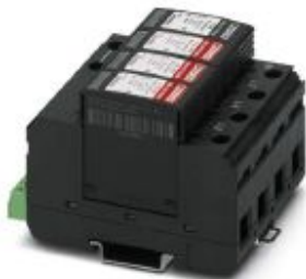
Surge voltage arrester 4-channel, for mounting on NS 35/7.5, with remote indicator contact. 230 V AC
