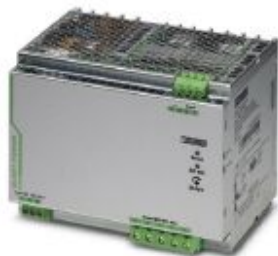
Primary-switched QUINT POWER power supply for DIN rail mounting with SFB (Selective Fuse Breaking) Technology, input: 1-phase, output: 48 V DC/20 A
