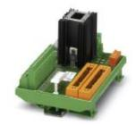
16-channel digital output module with screw connection and redundant voltage supply. Suitable for Yokogawa SDV 541 card.
