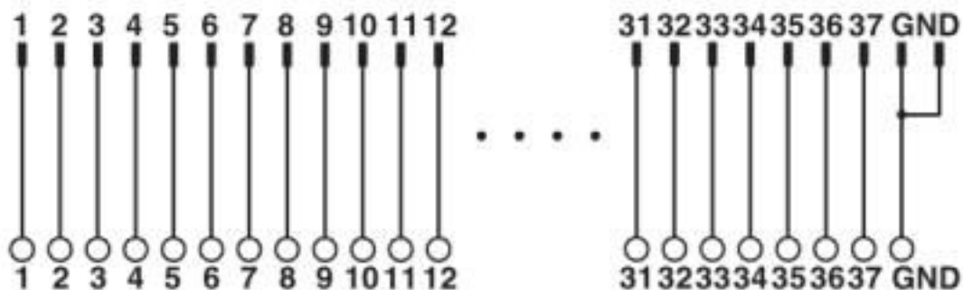
Connection scheme VIP-2/SC/D37SUB/M
