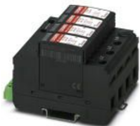
Surge voltage arrester combination 3-channel, for mounting on NS 35/7.5, with remote indicator contact as PDT, voltage 400 V AC
