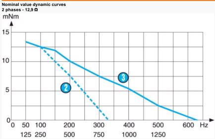
Measurement conditions : L 297298 SGS constant voltage supply board, 5.6 V at motor terminals, 2 phases energised, full steps, inertia of measuring system 4.53 g.cm2
