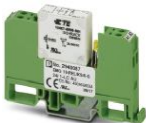
Relay module, with soldered-in miniature switching relay, gold contact for small loads, 1 N/O contact, input voltage 24 V DC
