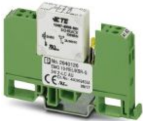
Relay module, with soldered-in miniature switching relay, gold contact for small loads, 1 N/C contact, input voltage 24 V DC
