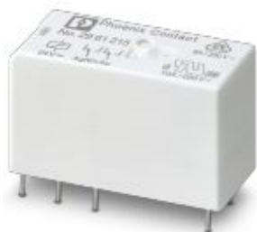
Plug-in miniature power relay, with multi-layer gold contact, 2 PDTs, input voltage 24 V DC
