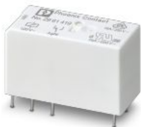
Plug-in miniature power relay, with power contact for high continuous currents, 1 PDT, input voltage 120 V AC
