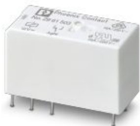
Plug-in miniature power relay, with multi-layer gold contact for high continuous currents, 1 PDT, input voltage 24 V AC
