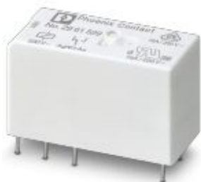
Plug-in miniature power relay, with multi-layer gold contact for high continuous currents, 1 PDT, input voltage 230 V AC
