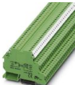
Power solid-state relay terminal block with short-circuit-proof DC voltage output, input: 24 V DC, output: 3 - 33 V DC/10 A
