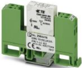
Relay module, with soldered-in miniature switching relay, gold contact for small loads, 1 N/O contact, input voltage 230 V AC/DC
