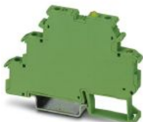
Power solid-state relay terminal block, input: 5 V DC, output: 10 - 253 V AC/800 mA, terminal block width: 6.2 mm
