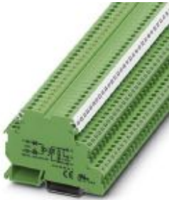
Power solid-state relay terminal block, input: 12 V DC, output: 10 - 253 V AC/800 mA, terminal block width: 6.2 mm
