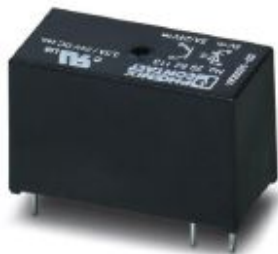
Plug-in miniature solid-state relay, power solid-state relay, 1 N/O contact, input: 5 V DC, output: 3 - 33 V DC/5 A
