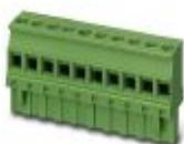
PCB connector, nominal current: 12 A, rated voltage (III/2): 320 V, nominal cross section: 2.5 mm<sup>2</sup>, number of positions: 20, pitch: 5.08 mm, connection method: Screw connection with tension sleeve, color: green, contact surface: Tin
