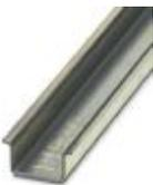
DIN rail, unperforated, Standard profile, width: 35 mm, height: 15 mm, similar to EN 60715, material: Steel, galvanized, passivated with a thick layer, length: 2000 mm, color: silver
