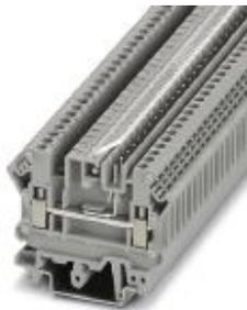
Feed-through terminal block, nom. voltage: 250 V, nominal current: 24 A, connection method: Screw connection, number of connections: 3, number of positions: 1, cross section: 0.2 mm<sup>2</sup> - 4 mm<sup>2</sup>, AWG: 24 - 12, width: 5.08 mm, color: gray, mounting type: NS 32, NS 35/15, NS 35/7,5
