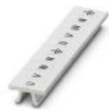
Zack marker strip, Strip, white, labeled, printed horizontally: U, V, W, N, GND, U, V, W, N, GND, mounting type: snap into tall marker groove, for terminal block width: 5.08 mm, lettering field size: 10.5 x 5.15 mm, Number of individual labels: 10
