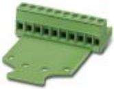
PCB connector, nominal current: 12 A, rated voltage (III/2): 320 V, nominal cross section: 2.5 mm<sup>2</sup>, number of positions: 11, pitch: 5.08 mm, connection method: Screw connection with tension sleeve, color: green, contact surface: Tin
