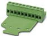
PCB connector, nominal current: 12 A, rated voltage (III/2): 320 V, nominal cross section: 2.5 mm<sup>2</sup>, number of positions: 9, pitch: 5.08 mm, connection method: Screw connection with tension sleeve, color: green, contact surface: Tin
