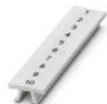
Zack marker strip, Strip, white, labeled, Printed vertically: consecutive numbers 1 ... 10, 11 ... 20, etc. up to 91 ... 100, mounting type: snap into tall marker groove, for terminal block width: 5.08 mm, lettering field size: 10.5 x 5.15 mm, Number of individual labels: 10
