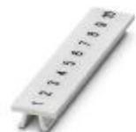
Zack marker strip, Strip, white, labeled, printed horizontally: consecutive numbers 1 ... 10, 11 ... 20, etc. up to 91 ... 100, mounting type: snap into tall marker groove, for terminal block width: 5.08 mm, lettering field size: 4.98 x 10.5 mm, Number of individual labels: 10
