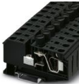
Spring-cage terminal block-fuse terminal block for cartridge fuse inserts with screw cap, cross section: 0.5 - 6 mm 2 , width: 12 mm, color: black
