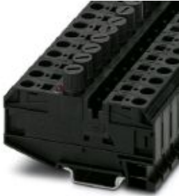
Spring-cage terminal block-fuse terminal block for cartridge fuse inserts with screw cap, cross section: 0.5 - 6 mm 2 , width: 12 mm, color: black
