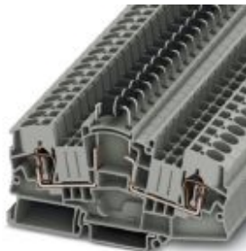
Component terminal block, with integrated P1000M diode, connection method: Spring-cage connection, cross section: 0.2 mm 2 - 10 mm 2 , AWG: 24 - 10, width: 8.2 mm, color: gray
