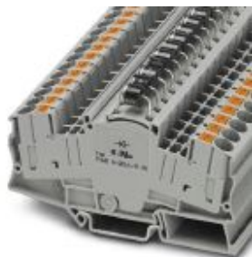
Component terminal block, with integrated P1000M diode, connection method: Push-in connection, cross section: 0.5 mm 2 - 10 mm 2 , AWG: 20 - 10, width: 8.2 mm, color: gray
