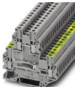
Protective conductor double-level terminal block, connection method: Screw connection, cross section: 0.14 mm 2 - 4 mm 2 , AWG: 26 - 12, width: 5.2 mm, color: gray, mounting type: NS 35/7,5, NS 35/15
