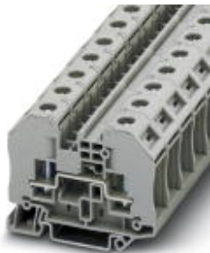
Thermoelectric voltage terminal block with bolt connection technology, cross section: 0.1 - 6 mm 2 , AWG: 26 - 10, width: 16.3 mm, color: gray
