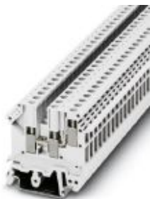
1-level terminal block with double connection on one side, cross section: 0.2 - 4 mm 2 , AWG: 24 - 12, width: 6.2 mm, color: White
