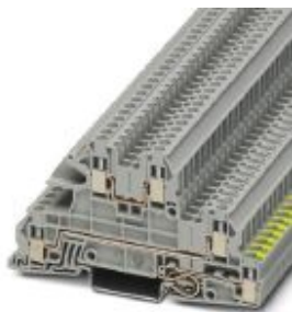
Installation ground terminal block, Screw connection, cross section: 0.2 mm 2 - 4 mm 2 , AWG: 24 - 12, width: 5.2 mm, color: gray, mounting type: NS 35/7,5, NS 35/15
