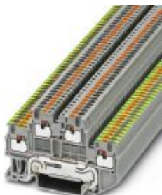
Protective conductor double-level terminal block, connection method: Push-in connection, cross section: 0.14 mm 2 - 1.5 mm 2 , AWG: 26 - 14, width: 3.5 mm, color: gray, mounting type: NS 35/7,5, NS 35/15
