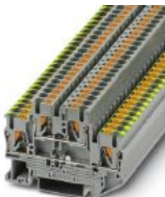
Protective conductor double-level terminal block, connection method: Push-in connection, cross section: 0.14 mm 2 - 4 mm 2 , AWG: 26 - 12, width: 5.2 mm, color: gray, mounting type: NS 35/7,5, NS 35/15
