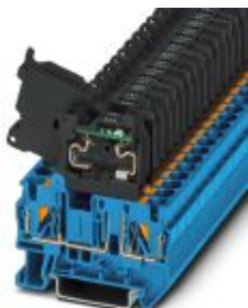
Lever-type fuse terminal block, with blue basic terminal block and black lever, for 5 x 20 mm cartridge fuse-links, with LED for 24 V DC
