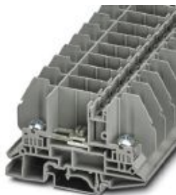
Feed-through terminal block with bolt connection, cross section: 0.1 - 6 mm 2 , AWG: 26 - 10, width 16.3 mm, color: Gray
